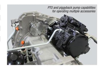
Functional Concept Note: The HydroMech iVT features a hydrostatic drive at low speeds for improved vehicle control; synchronous shifting from variator drive to 1st powersplit gear; and powershift clutching from 1st powersplit gear to 2nd with variator gap compensation.
