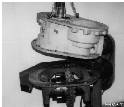
Picture 14: Removal of the spur gear housing
