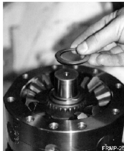
Picture 27: Installation of the adjustment shim underneath the bearing
