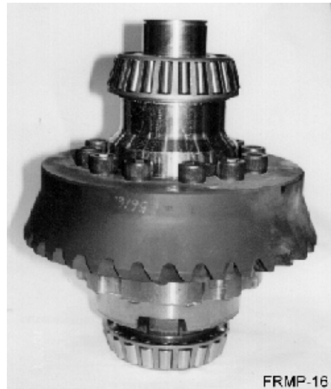
Picture 19: Differential unit with the crown wheel; the engagement ring for differential lock and the locking ring are removed
