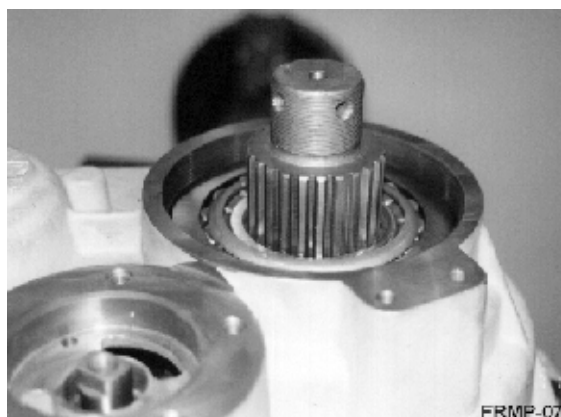
Picture 9: Input bearing adjustment nut removed and housing ready for dismantling
