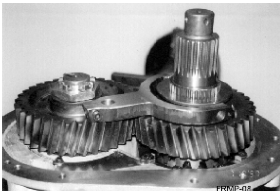
Picture 30: Assembled spur gear unit, but without the outer bearing
