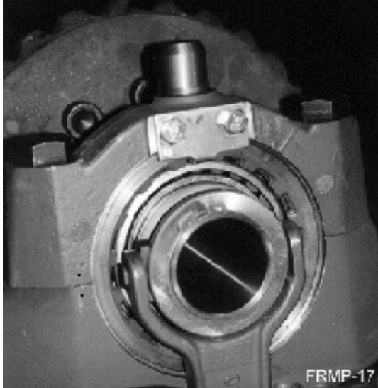
Picture 18: Differential unit and bearing cover marking before dismantling
