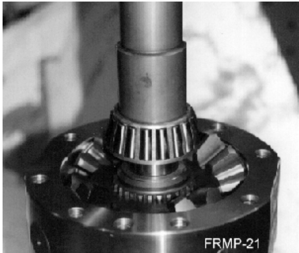
Picture 28: Installation of the inside tapered roller bearing cone
